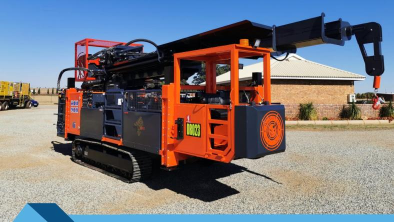
Heavy duty Track or Truck mounted, for Reverse Circulation or Grade. Control Supplied complete with basic set equipments, including on board Air Compressor.
